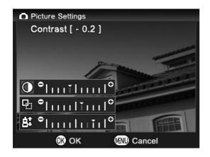
Use the \$\rightharpoonup \text{arrows on the 4-way controller to select [Contrast], [Saturation], [Sharpness] from [Picture Settings], then press the \$\rightharpoonup \text{ arrows on the 4-way controller to adjust the compensation.} Press the \$\rightharpoonup \text{ button to apply the setting or the MENU button to close the sub-menu without making any changes.}
