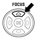
When setting AF mode to normal autofocus (without an icon), the focusing distance is from 28cm to infinity. It is possible to change AF mode to LIMIT mode ( is displayed) by pressing the **FOCUS** button. In LIMIT mode, the focusing distance will be from 1m to infinity and the AF speed will be faster.
