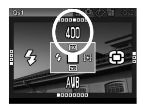
For example, if you wish to change the ISO Setting to 400, press the QS button to display Qs1, then set the value to 400 by pressing the
