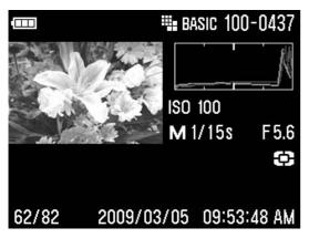
This histogram shows that many of the pixel values are at their brightness limit, indicating that some areas of the image may be blown out. In general, when the histogram runs off the right side, the image will have many white pixels—either because the image is overexposed or because it is a bright scene such as the beach or snow.
