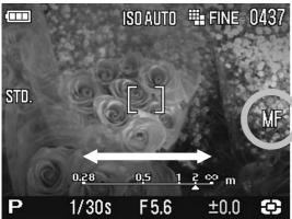
In situations where autofocus or focus lock is not effective, you can focus manually.
