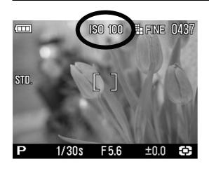
The photosensitivity of digital cameras is described in terms of "ISO equivalent" like silver-halide film cameras. (ISO sensitivity **P.112**)
