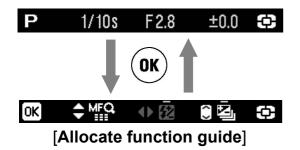
During the Shooting Mode, it is possible to change the exposure indicator at the bottom of the display to the Allocate function guide by pressing the (IK) button. It is possible to confirm the current allocated function by pressing the (\$\Display\$) button and the \$\Display\$ button.
