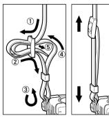
Undo both ends of the supplied strap and attach it to the right and left strap holders as shown.
